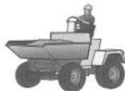
DUMPER Capacity: ~0.3 to 0.75m 3
