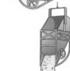
ROLLOVER SKIP Capacity: ~0.2 to 1.0m 3
